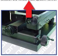
CheckMate manual stations utilize coaxial coarse and fine drive knobs for the utmost in control and convenience. As your needs change, so can your prober, In Your Lab!
